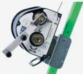
8510224 WINCH/SRL MOUNTING BRACKET FOR 8513158 TRIPOD Attaches to the leg tube with quick-release pins for tool-less set-up and adjustment. Weight: 3 lbs. (1.4kg)
