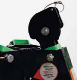
8512293 TOP PULLEY ASSEMBLY FOR UCT SERIES TRIPODS Pulleys are mounted on top of the head assembly to route mechanical device's lifeline over and into confined space area. Weight: 1.6 lbs. (.73kg)
