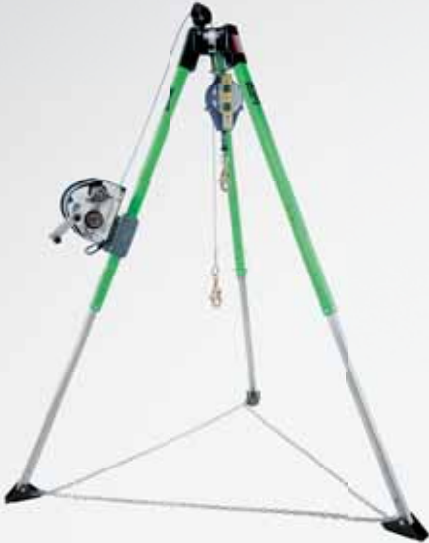
8513158 ADVANCED UCT-300 7' (2.13m) TRIPOD Lightweight, durable aluminum construction with powder coat finish Includes quick connect winch mount bracket – can accommodate up to three brackets Includes top mounted pulley system – can accommodate up to three pulleys Telescoping adjustable locking legs for easy set-up Fast detent pin style adjustment and locking Inner plastic liners provide smooth adjustment Foot pads include sharp points for biting into soft ground and/or uneven terrain Safety chain for added support, strength and safety 5,000 lb. (22kN) built-in head-mounted anchor point
