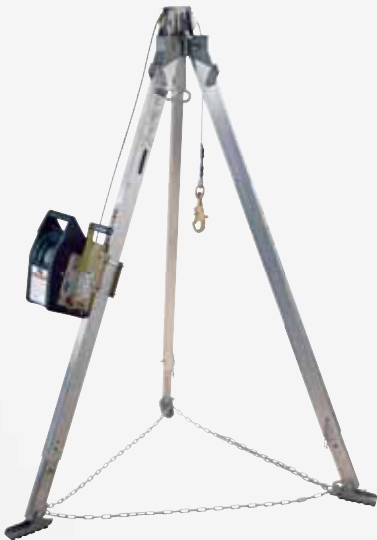
8000000 ADVANCED 7' (2.13m) ALUMINUM TRIPOD Lightweight, durable aluminum construction Includes quick connect winch mount bracket Includes top mounted pulley system Telescoping adjustable locking legs for easy set-up Fast detent pin style adjustment and locking Rubber safety shoes with spiked edges for different terrains Safety chain for added support, strength and safety 5,000 lb. (22kN) built-in head-mounted anchor points
